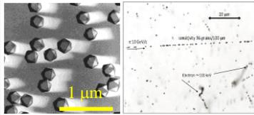
Fig. 2. Left: AgBr crystals in emulsion layers observed by SEM. Right: A minimum ionizing track (MIP) of a 10 GeV/c pion.
