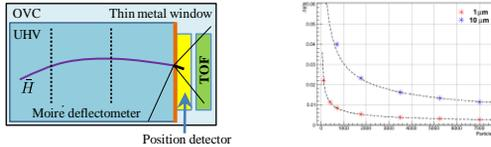
Fig. 1 Left: Schematic view of the AEGIS detectors. Right:  $\Delta g/g$  vs. number of particles for a position sensitive detector resolution of 1  $\mu\text{m}$  (red) and 10  $\mu\text{m}$  (blue).
