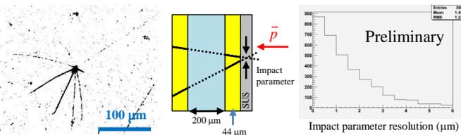
Fig. 6. Left: A typical antiproton annihilation vertex in the emulsion layer. Middle: Definition of the impact parameter. Right: Impact parameter resolution with a window of 20  $\mu\text{m}$  stainless steel (SUS).
