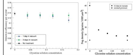
Fig. 4. Left: Crystal sensitivity vs. glycerine concentration. Right: Fog density vs. glycerine content for films kept in vacuum for 3.5 days (square), compared to atmospheric pressure (dots).
