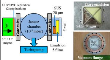
Fig. 5. Left: Schematic view of the detector setup. Upper right: Emulsion holder. Lower right: Emulsion detector attached to the vacuum flange by a crossed bar frame.
