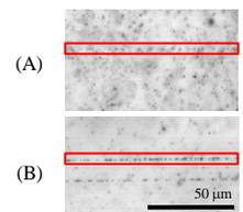
Fig. 8. A 10 GeV/c pion track in the reference film (A) and in a highly sensitive one (B).
